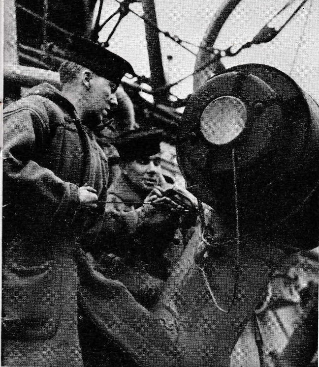
The depth charge thrower was the main anti-submarine weapon of World War II. The depth of the target had to be estimated and the setting on the charge made by hand. It was not an accurate weapon.
